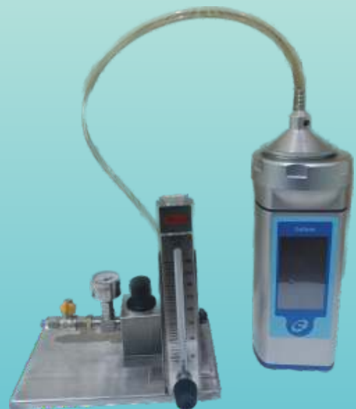
Compressed Air Assembly
